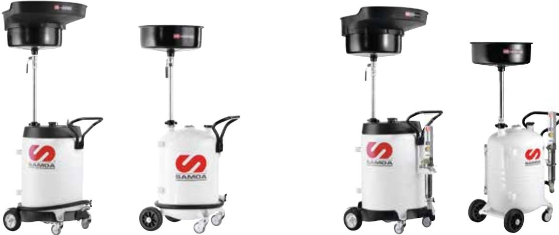
**Gravity collection with pressure discharge.** Discharge is done through a 1,5 m hose pressurizing the unit at 0,5 bar (3.5 psi). Includes a safety valve to avoid over pressurization.
